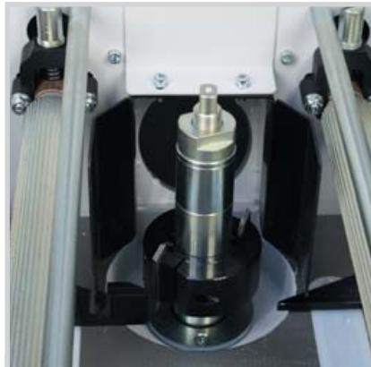
Vertical spindle. Max moulding height 130 mm.
