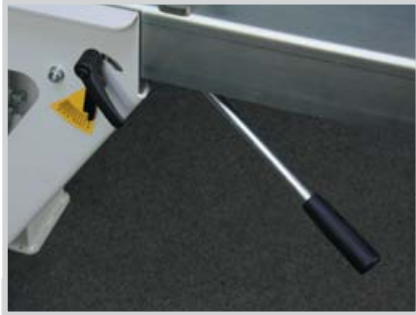
Planer cut depth is easy to adjust between 0 - 10 mm.
